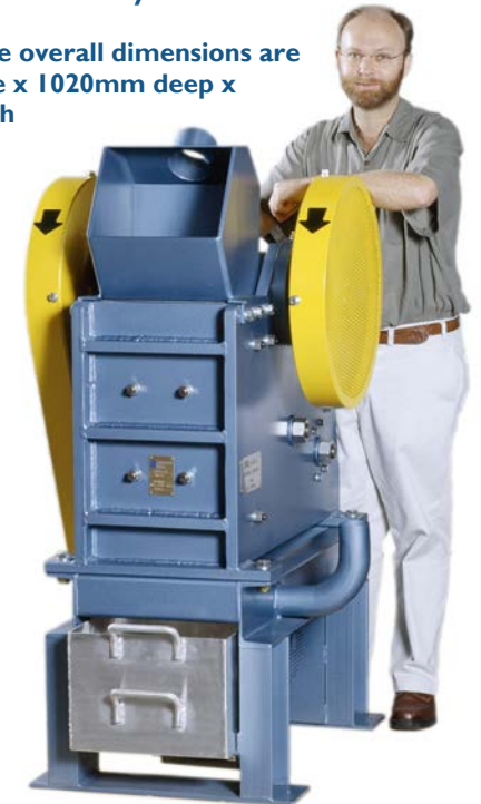
Typical JC3000 configuration for stand alone analytical or metallurgical laboratory use
